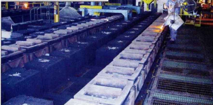
While several jolt-squeeze machines are still in use, the two newer automatic mold lines do the heavy lifting in meeting the quick turnarounds. Patterns are changed as many as 15 times a day on each molding line.
