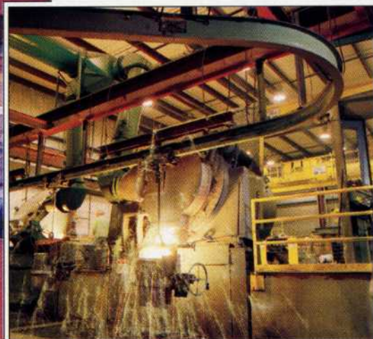
Gartland eliminated its cupola in 1995 when it chose electric melting for better flexibility and efficiency. The new building (featuring a poured concrete basement for water and controls) includes two coreless induction furnaces that can supply iron at a rate of 5 tons/hr.
