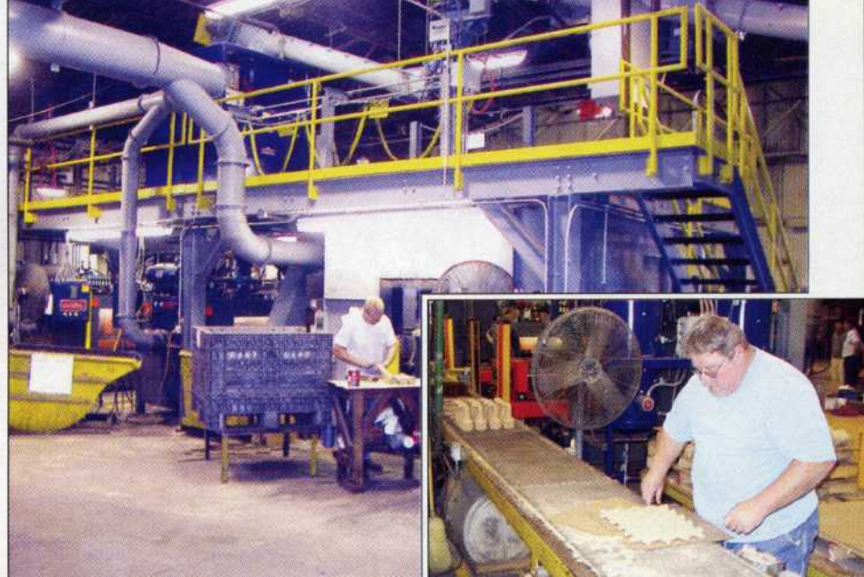
A $500,000 coreroom modernization was completed in July, which added two new core machines, a mixer, amine supply system, scrubber, sand heater and conveyor.
